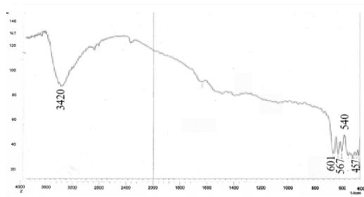
Fig. 4. FTIR transmittance spectrum of In_2O_3 at (600\text{ }^\circ\text{C}) as a function of wavenumber
