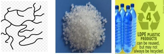
Fig. 2. Polyethylene low density, inner structure, applications
