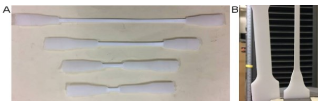
Fig. 7. Polycarbonate and polyethylene low density under test stage
