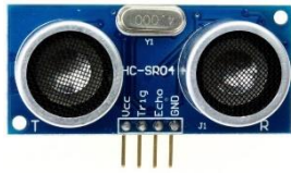
Fig. 3. Example of HC-SR04 ultrasonic sensor
