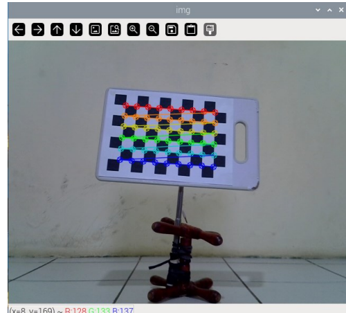
Fig. 3. Camera calibration process display
