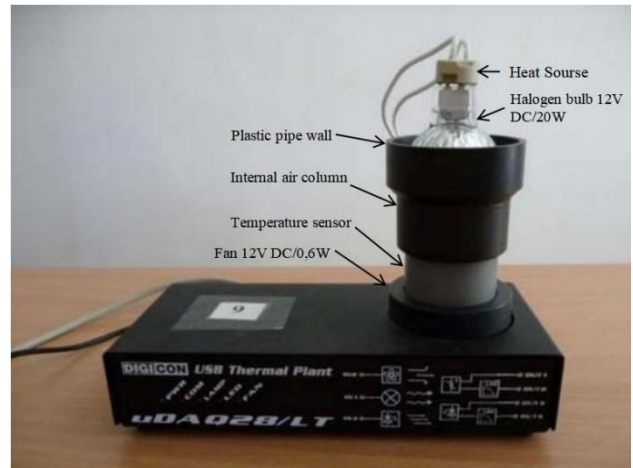
Fig. 5. The combined thermo-optical laboratory plant (uDAQ28/LT) [5]
