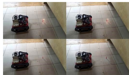
Fig. 18. Successful Fire Extinguishing Using Powder by The Robot
