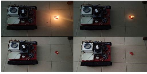
Fig. 19. Successful Fire Extinguishing Using Water by The Robot
