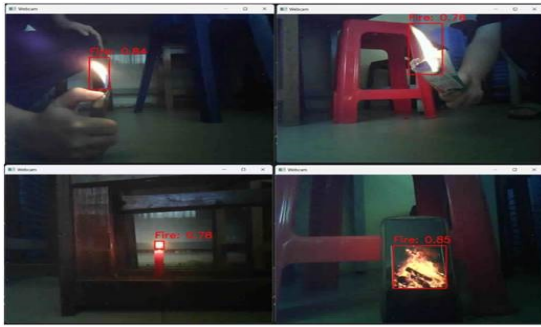
Fig. 16. Detection of Various Types of Flames
