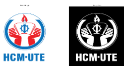
Fig. 4. Image output after scaling and binary conversion
