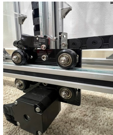
Fig. 5. Z-axis movement mechanism
