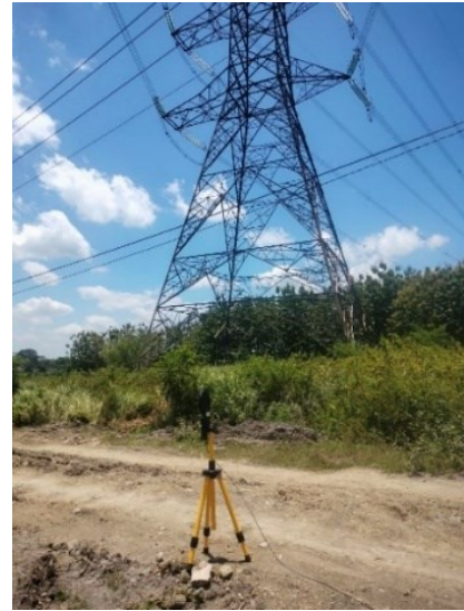
Fig. 4. Experimental setup for EF measurements using the ETS-Lindgren HI-3604 ELF Survey Meter
