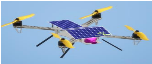
Fig. 1. Solar cell small drone self-feeding battery
